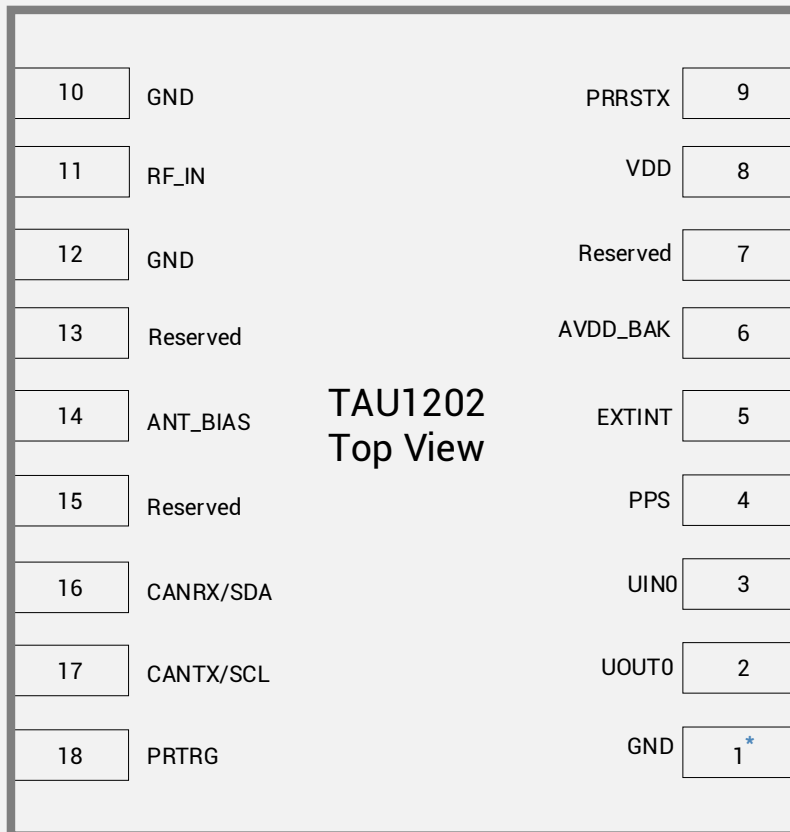
Figure 3 Pin assignment (top view)
